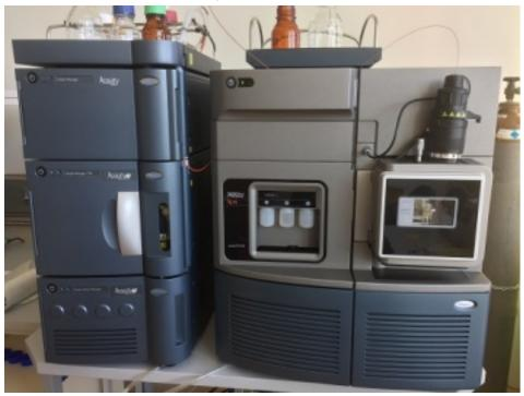
This instrumentation will form the instrumental basis of our Analytical Laboratory and will be used primarily for targeted, highly sensitive quantification of substances. The cell consists of two main modules. The Acquity ultra performance liquid chromatograph (UPLC) module and the Waters Xevo TQ-XS tandem mass spectrometer (MS).
