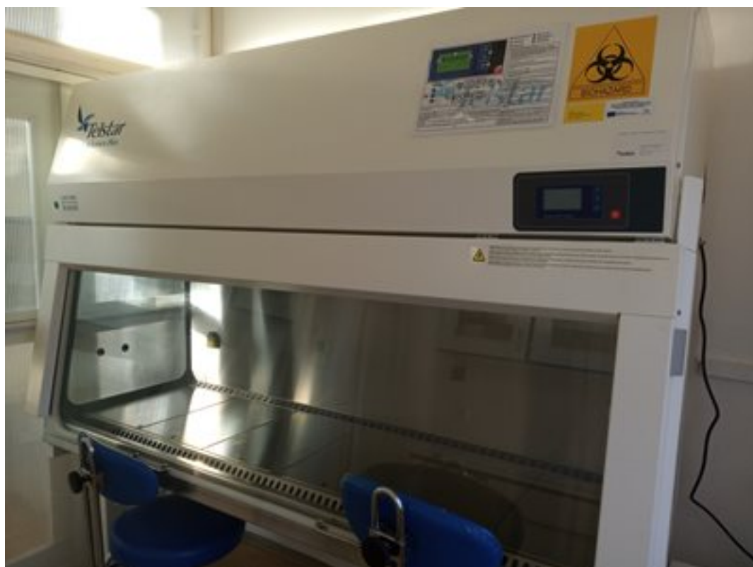
Photo 2: Biohazard box with laminar flow featuring two workstations, allowing two students to work simultaneously. During the CA, cells are placed in an agarose gel. After lysing the cell and nuclear membranes in a salt solution, DNA fragments migrate out of the nucleus, more precisely from the nucleoid ("head") to the "tail" due to electrophoresis, creating the characteristic comet image after visualization with a suitable dye, which gives the method its name. The
